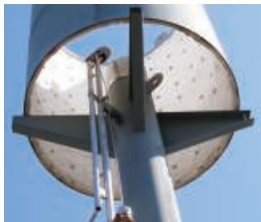
FIGURE 8. Shown here (above left and top) is a small, elevated enclosed flare that operates in a “smokeless,” air-assisted type
