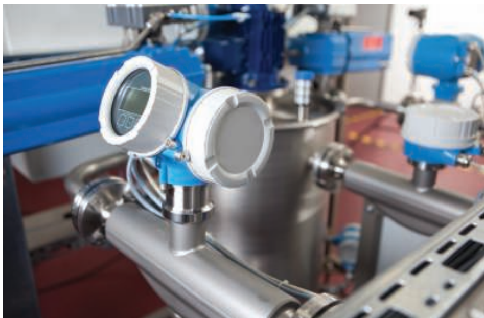
FIGURE 1. Flowmeters like the one shown here can play key roles in reducing risks with safety instrumented systems (SIS)
