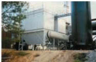
FIGURE 2. The image at left shows two baghouses installed in parallel. On the right, the cage is inserted into filter bags, and pulse-jet pipes provide blowback to clean the dust off the filter
