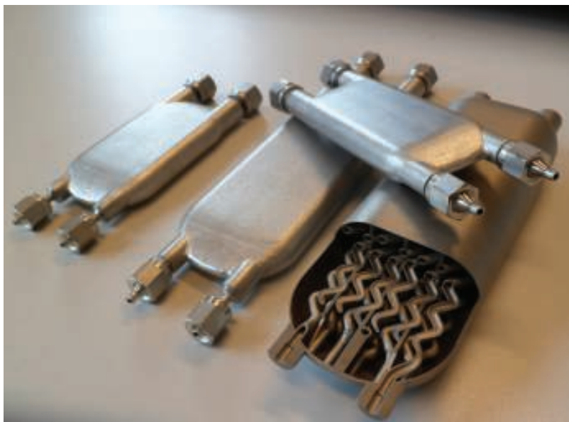
FIGURE 8. These flow-reactor modules were manufactured by 3-D metal printing
